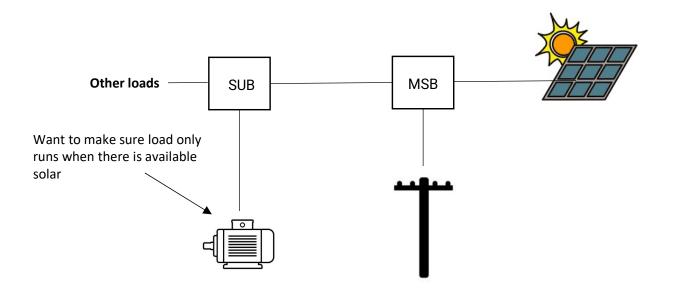
You only want to turn the motor load on and off based on solar exports, so you cannot switch the submain from the Main Switchboard.
