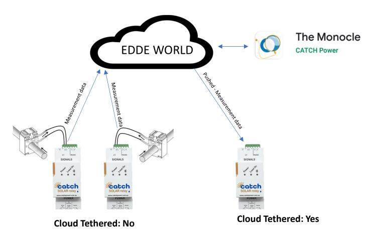
These devices use the CT readings to perform load control and inverter control. The measured data is sent to the EDDE WORLD This devices uses the measurement data from EDDEWORLD to perform its load control and inverter control operations.
