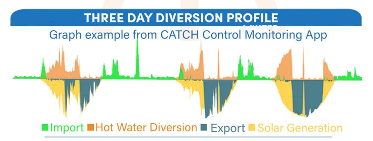
Even though Green CATCH has no monitoring you can see the effects of Green CATCH working. The cunsumption profile perfectly mirrors the solar production. This energy would otherwise be sent to the grid.
