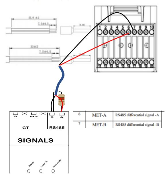
Ensure the data cable is rated for the voltages it will be in close proximity to. A 120 Ohm terminating resistor may be required at the CATCH Relay terminals as shown in the diagram below if the cable run is longer than 10m.
