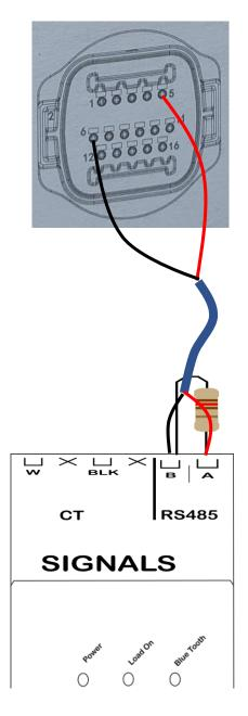
Ensure the data cable is rated for the voltages it will be in close proximity to. A 120 Ohm terminating resistor may be required at the CATCH Relay terminals as shown in the diagram below if the cable run is longer than 10m.
